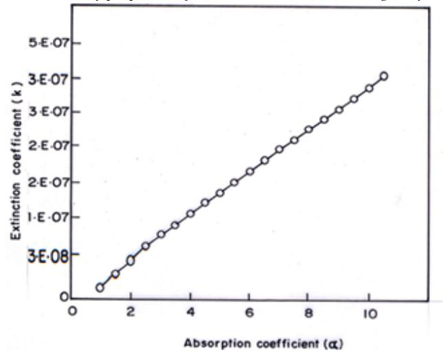
FIGURE 4. Plots of extinction coefficient ( $K$ ) vs absorption coefficient ( $\alpha$ ).
