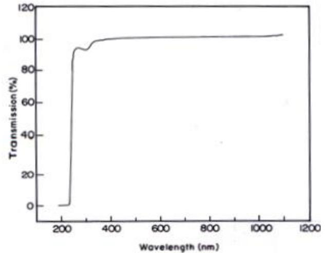
FIGURE 1. Transmittance spectrum of LHN.
