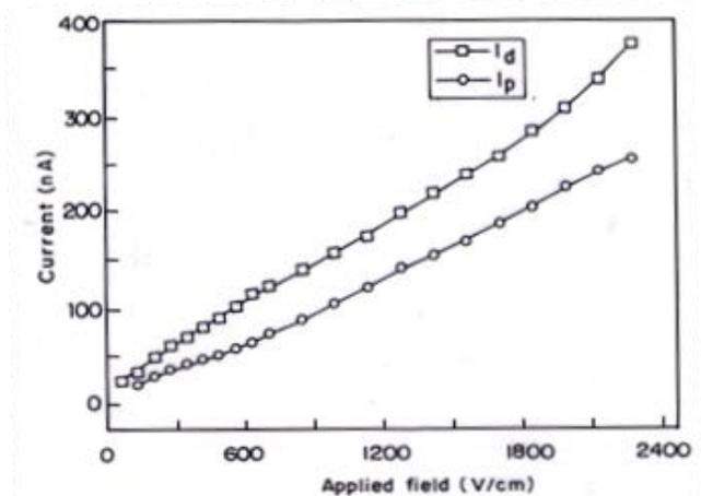
FIGURE 7. Field dependent photoconductivity of LHN single crystal.
