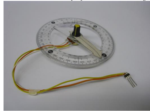
FIGURE 8. The proposed apparatus to generate different output signals. The potentiometer is centered in the protractor and it has three wires to connect a parallel resistor, according to the Figs. 9 and 12 circuits.
