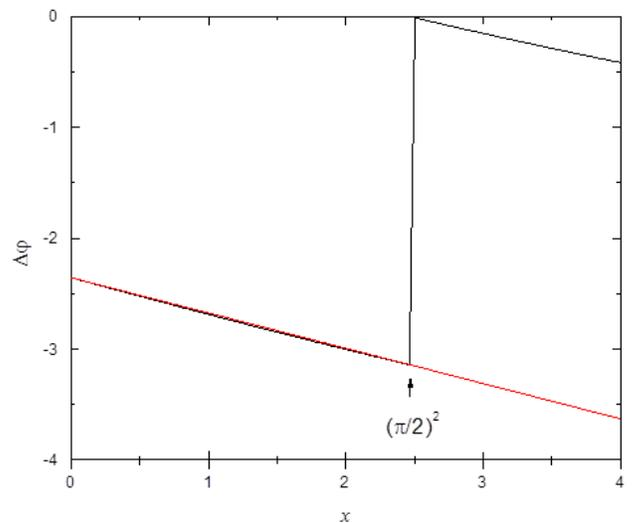
FIGURE 2. Phase lag vs  $x = f/f_c$ . Eq. (2) is represented by the black line and Eq. (19) by the red line.
