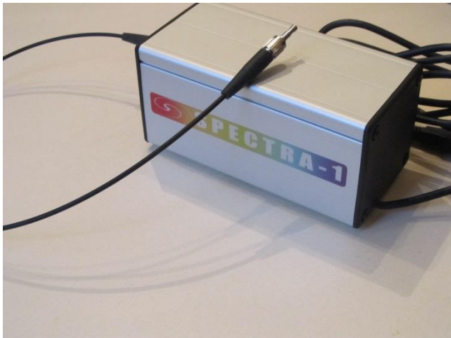
FIGURE 1. A picture of the compact digital spectrophotometer employed in the present investigation (3BScientific, Mod. U17310), showing also the optical fiber through which the light enters into the device.
