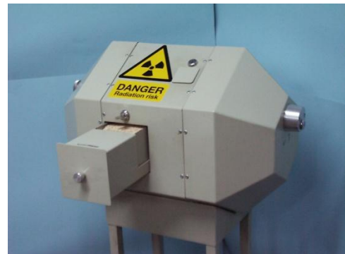
FIGURE 1. Measuring shielded head for neutron experiment in teaching.
