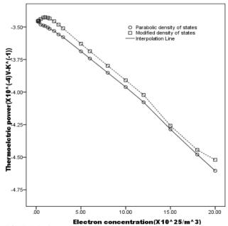
**FIGURE 1.** shows thermoelectric power as a function of electron concentration with the solid line marked by circles is for parabolic band case and dashed line marked by squares is for modified density of states.
