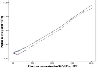
**FIGURE 2.** shows Peltier coefficient as a function of electron concentration with the solid line marked by circles is for parabolic band case and dashed line marked by squares is for modified density of states.
