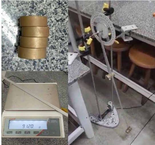
FIGURE 4. Set of materials used in the experiment: cylinders, metal bar and fixing elements. Regarding the measurement of periods, the sensor indicated the time interval of each oscillation.
