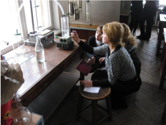
FIGURE 10. Students performing the Alexander’s diving bell experiment to measure the acceleration of gravity.
