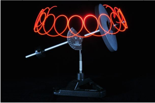
FIGURE 5. Precession and nutation pattern for z_{cm} < 0 when the axis is released with horizontal backward impulse ( \dot{\theta}(0) = 0 , \dot{\phi}(0) > 0 ). Exposition time is 17.15s.
