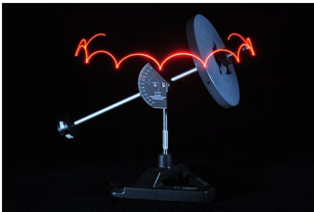
FIGURE 6. Precession and nutation pattern for z_{cm} < 0 when the axis is released from rest ( \theta(0) = \dot{\phi}(0) = 0 ). Exposition time is 14.2s.
