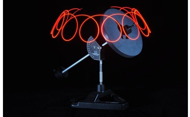
FIGURE 7. Precession and nutation pattern for z_{cm} < 0 when the axis is released with horizontal backward impulse ( \dot{\theta}(0) = 0 , \dot{\phi}(0) > 0 ). Exposition time is 14.5s.
