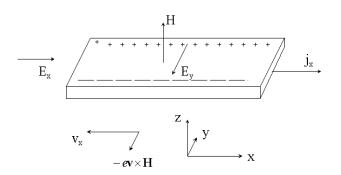
FIGURE 1. Schematic of Hall effect experiment. Usually the electric carriers are believed to be electrons. The electrons move against the external electric field and therefore, Lorentz force make them move toward downside. The resultant electric field is along -y direction resulting in negative Hall coefficient.
