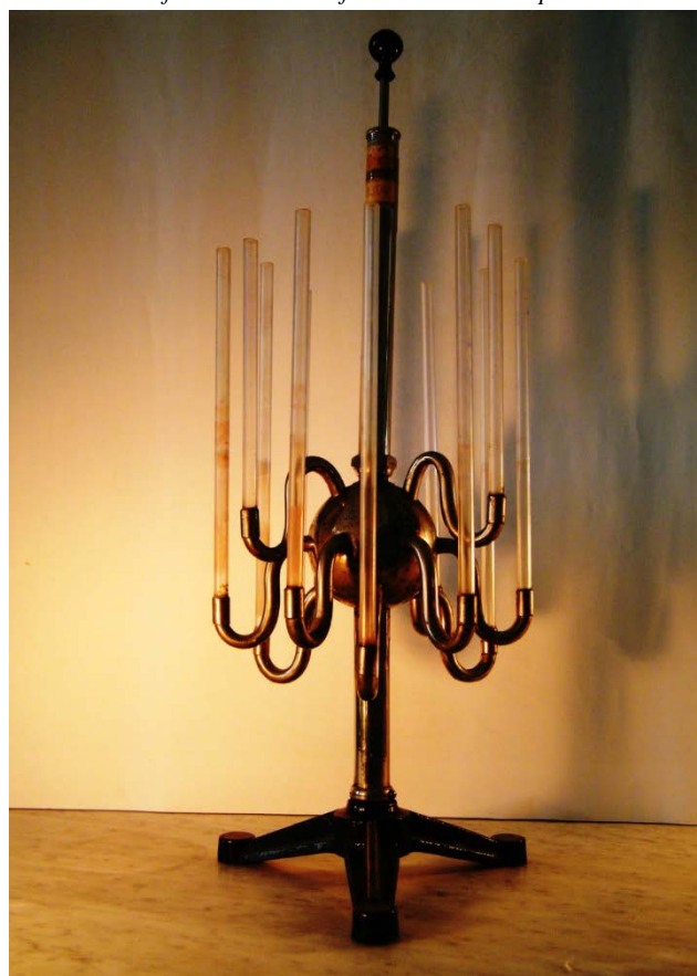
FIGURE 4. Demonstrator of Pascal law. This apparatus has 12 manometers and the height is about 540 mm. The apparatus is made using chromium plated brass. The realization date is the beginning of the twentieth century.
