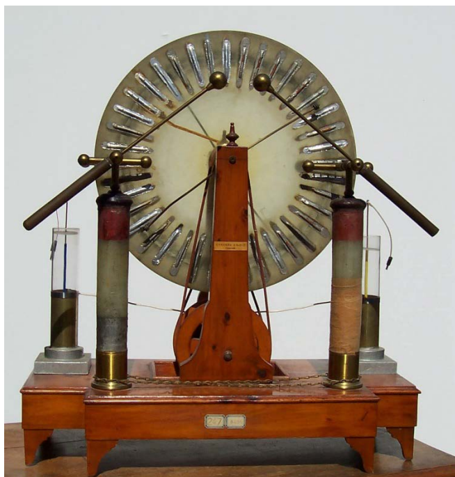
FIGURE 3. A beautiful electrostatic machine signed "Egidio Caranza" probably manufactured at the end of the XIX century. The dimensions of this beautiful apparatus are Length 700 mm; width 335 mm; height 750 mm. Disks' diameter 470 mm. Two Leyden jars were added in the half of XX century. In Chiavari we found other two electrostatic machines of this craftsman.
