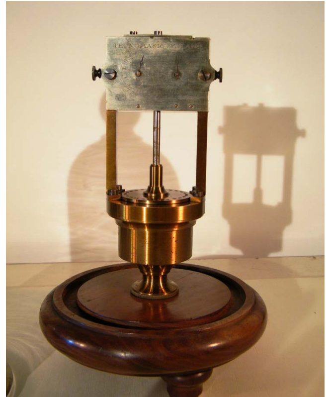
FIGURE 2. The siren made "Tecnomasio - Milan".
