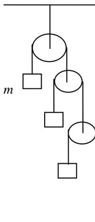
FIGURE 5. An infinite Atwood's machine.
