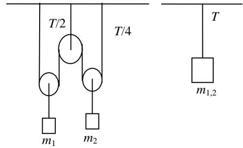
**FIGURE 11.** a) A system including the  $m_1$  and  $m_2$ . b) An equivalent system for (a).
