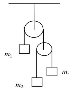
**FIGURE 4.** An Atwood's machine in series.
