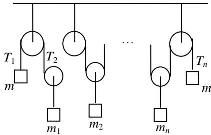
**FIGURE 7.** A parallel network for  $m_1, m_2, \dots, m_n$  and  $T_1 = T_2 = \dots = T_n$ .
