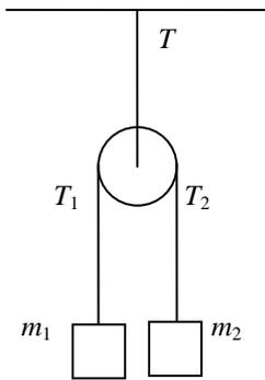
**FIGURE 2.** A simple Atwood's machine, that it consisting of two suspended masses connected by a string that passes over a pulley.
