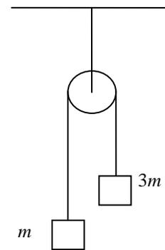
FIGURE 6. Equivalent system for Fig. 5, the acceleration of  $m$  is  $g/2$ .
