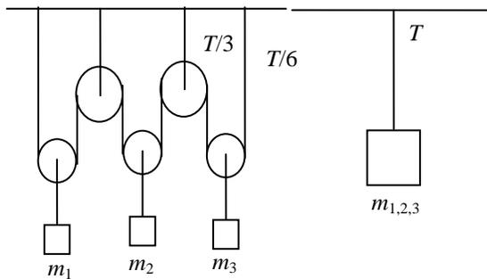
FIGURE 14. a) A system including  $m_1, m_2, m_3$  b) An equivalent system for (a).
