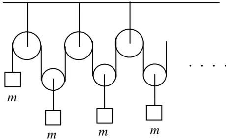
FIGURE 18. An infinite Atwood's machine.
