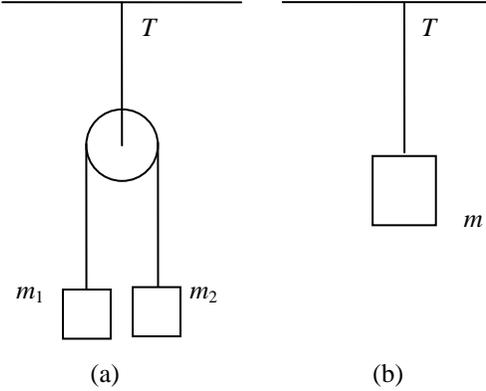
**FIGURE 3.** An Atwood's machine (a) and equivalent system for it (b).
