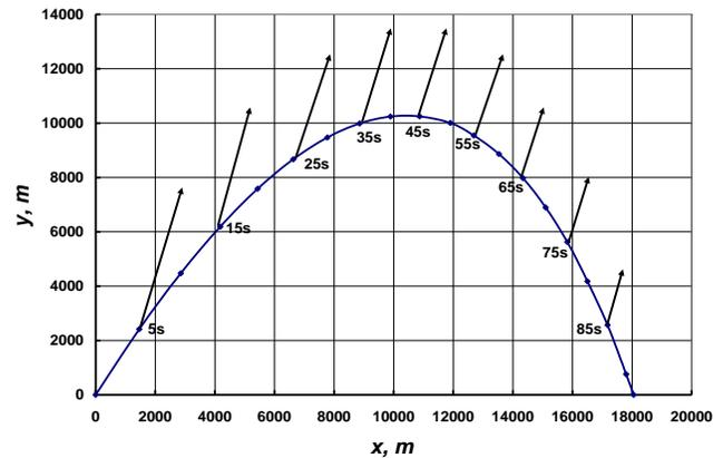
FIGURE 2. The jerk vector in projectile motion with launch speed  $v_0 = 600\text{m/s}$ ; launch angle  $\alpha = 60^\circ$ ; and drag coefficient  $k = .01/\text{s}$ .
