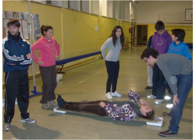
FIGURE 2. The "E. Fermi" High School of Ragusa students measure the human body barycentre position.
