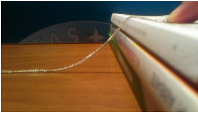
FIGURE 2. a) A small necklace of length L lies over the vertical profile of a pile of books, the remaining part lies on a horizontal surface. The end of the vertical portion is held by a finger at the edge of the step. b) The string is slowly dragged by the finger over the pile of books, while the other end is not moving: the suspended part of the string is seen to take the form of a catenary.
