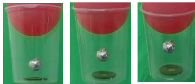
FIGURE 4. In free fall, the aluminum sphere gets closer to the balloon.
