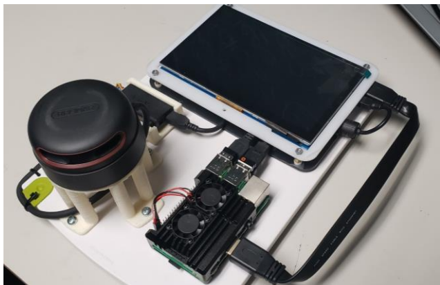
FIGURE 1. RPLIDAR A2 Connected to a RASPBERRY 3b+.
