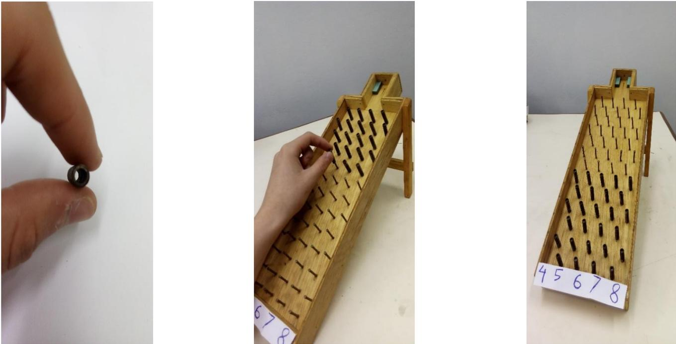
**FIGURE 1.** Our Galton board with 12 effective lines and 5 columns ending in bins that collect marbles. The choice of numbering for the bins follows the standard of traditional broad boards (not limited by walls). On the left, one can see the removable sleeve that turns the nails into screws.
