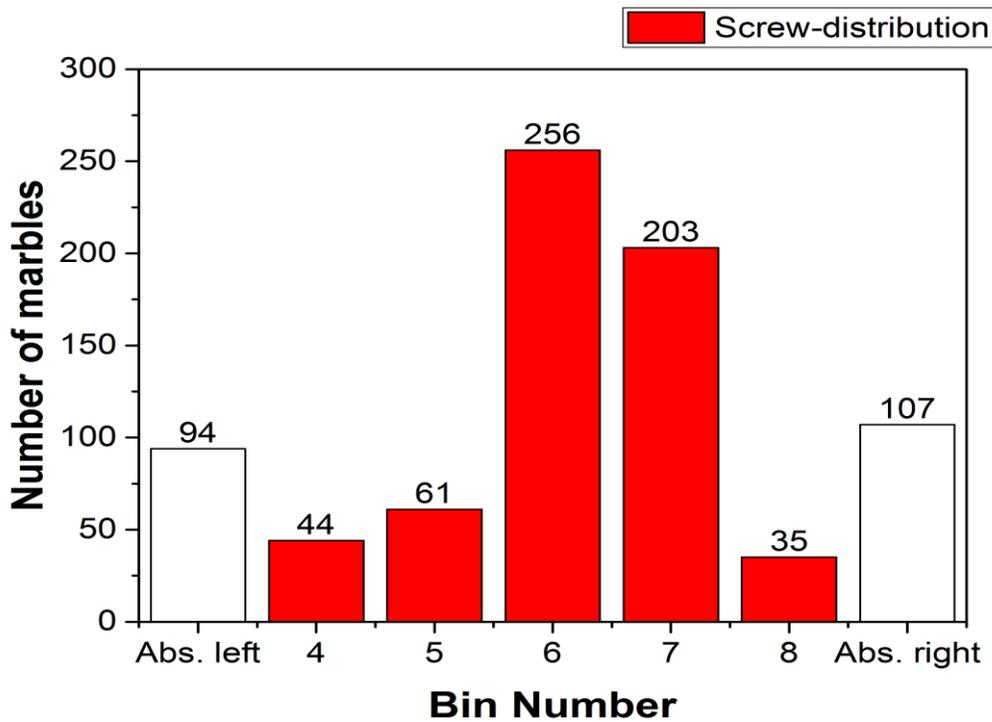
FIGURE 3. The experimental distribution of 800 marbles in the five bins in our Galton board with screws. The colorless columns show absorption on the left and right walls.
