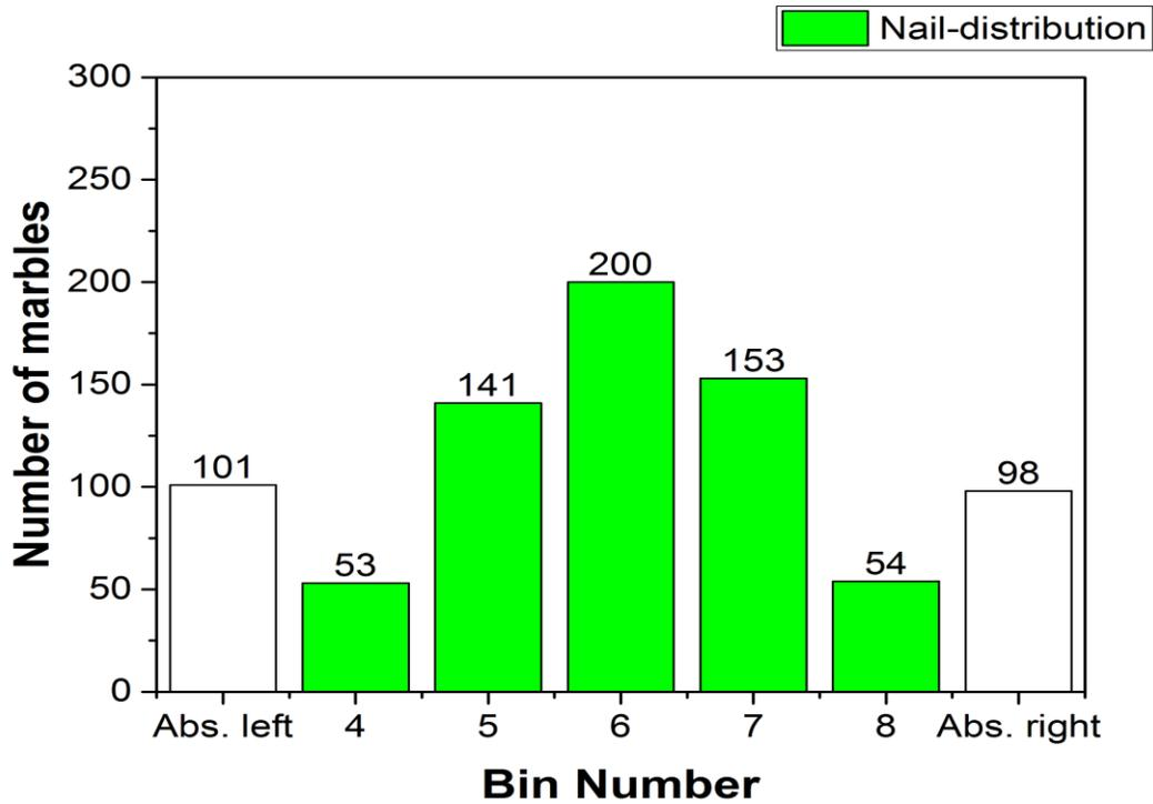
FIGURE 2. The experimental distribution of 800 marbles in the five bins in our Galton board with nails. The colorless columns show absorption on the left and right walls.
