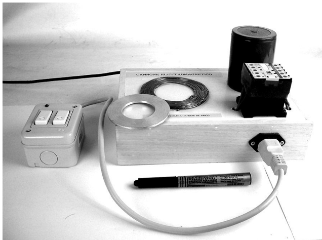
FIGURE 7. The Electromagnetic Cannon. The aluminium disk is shown displaced to view the coil. The capacitor is the large black cylinder and the contactor is in the right foreground. The remote control is on the left.
