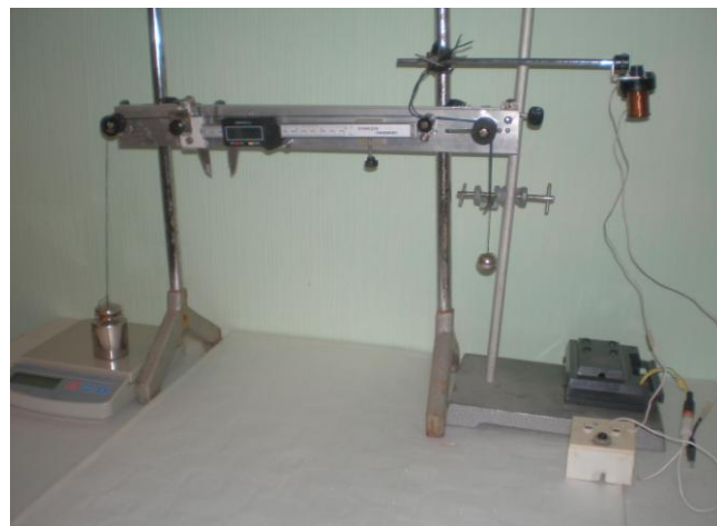
FIGURE 7. Experimental setup to determine Q factor of a simple pendulum.
