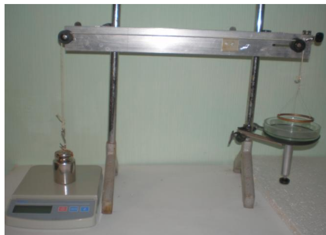
FIGURE 4. The experimental installation for determination of surface tension of liquids.
