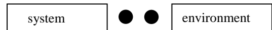
FIGURE 1. The superblock configuration: two blocks and two sites to add at each step of the DMRG procedure.
