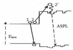
**FIGURE 7**. A representation of the Auger process.
