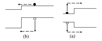
**FIGURE 2.** A representation of energy up-conversion for a) type-I heterostructure b) type-II heterostructure.
